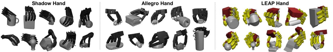
Fig. 5: Visualization of some grasps in our large-scale simulation evaluation. The evaluation totally involves 15k grasps on 478 objects and three dexterous hands. These figures show the grasp states after lifting from a table, achieved using our approach.
